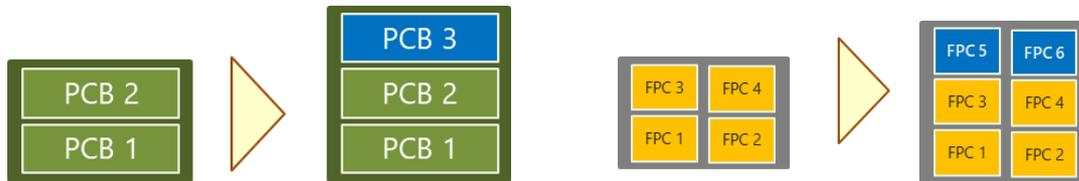
Figure 2a and 2b. Dual 330mm rails increase board and carrier capacity per lane.
